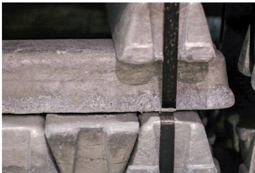
Corrosion resulting from water contact
