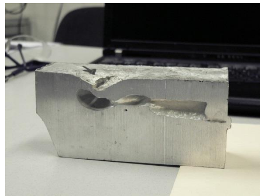
Surface porosity connected to large voids
