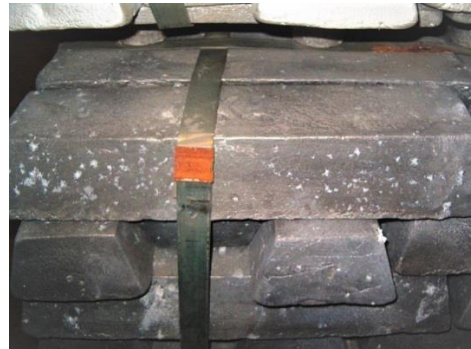
High concentration of corrosion spots
