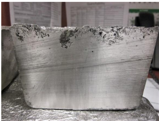
High concentration of sub-surface oxides
