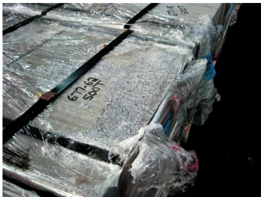
Corrosion due to trapped moisture
