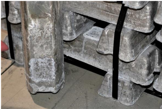
Excessive surface corrosion
