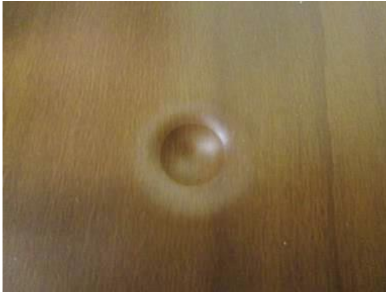
Photo No. 13 Typical Impact Dimple Detail (Exterior)
