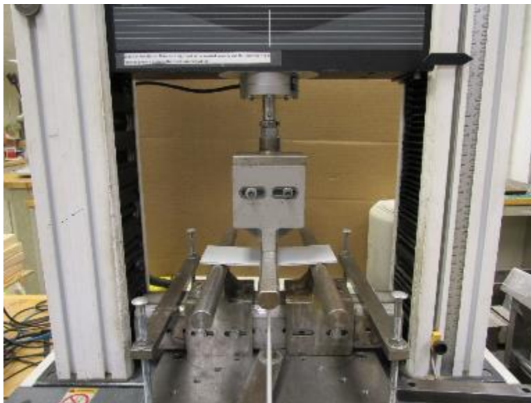
Photo No. 8 Typical Flexural Test Setup Detail
