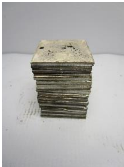
Photo No. 26 Typical Post-Test Combustion Specimen Detail
