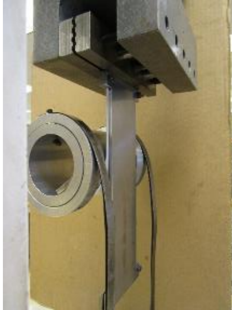
Photo No. 5 Typical Climbing Drum Peel Test In-Progress Detail
