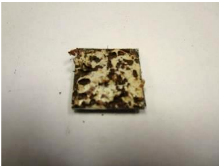
Photo No. 18 Typical Post-Test Ignition Specimen Detail
