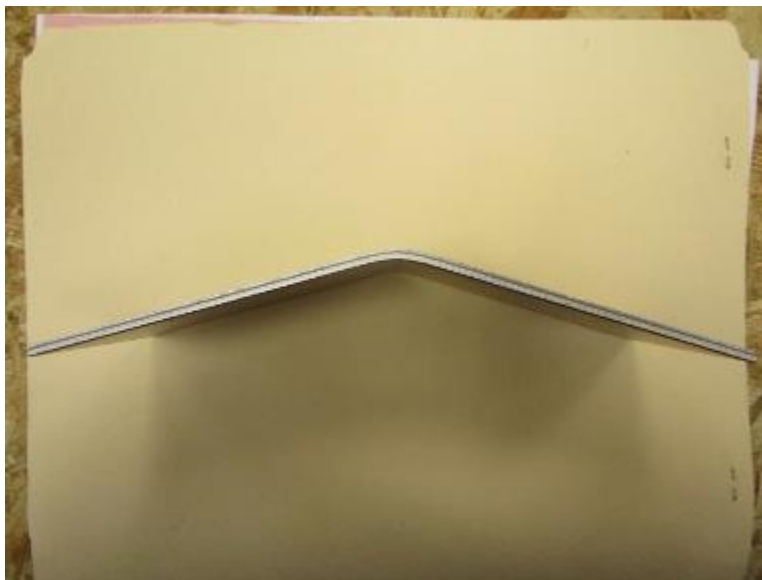
Photo No. 10 Typical Post-Test Flexural Specimen Detail
