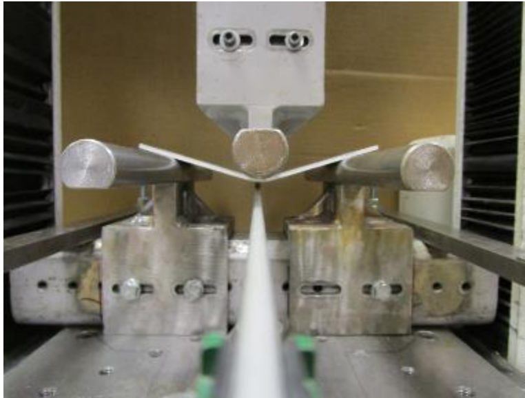
Photo No. 9 Typical Flexural Test In-Progress Detail
